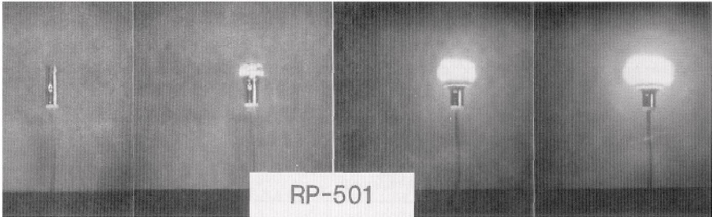
*RP-501 Detonation: A high speed camera has captured the detonation at 4 microsecond intervals*
